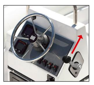
Control mounts on starboard <u>side of console</u> (as shown above) with right hand thumb trim actuation.
